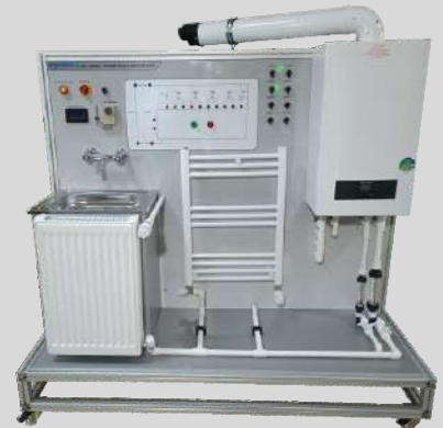
H-961 GAS COMBI FAILURE TRAINING SET
