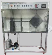
K-212 HEAT RECOVERY TYPE AIR CONDITIONING T.S
