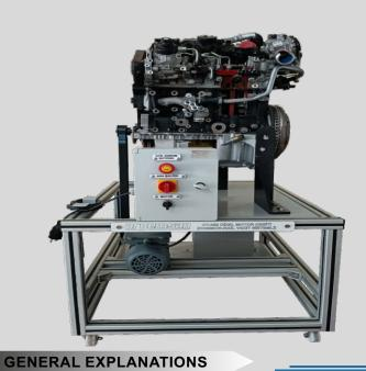
This training set is common-rail diesel engine with a fuel system show the working principle prepared for the purpose.
